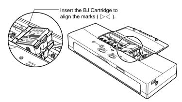
**6.** Press down gently on the high side of the BJ Cartridge until it snaps in place.
